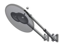
2. Attach arm to swivel ball on hub
